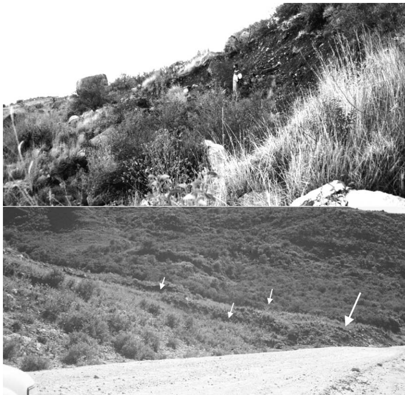
Fig. 9. Slump on the northern slope of Amba Raesat ((C) on Fig. 3) (photographs: February 2000). The upper image shows the slump head in weathered Amba Aradam sandstone colluvium and marl belonging to the upper Antalo limestone. The person is standing at the slide head, on the junction between the main scarp and the slide plane, roughly parallel to the surface, sloping with a gradient of 0.56 \text{ m m}^{-1} . The bottom picture shows the slump toe (white arrow) after cleaning of the 12-m wide road (foreground). The slumped mass is dissected by gullies (smaller arrows). The slope gradient here approximates 0.2 \text{ m m}^{-1} .
